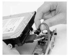
5. Connect both power and SATA cable from Base Plate bridge into the back of SATA hard drive
